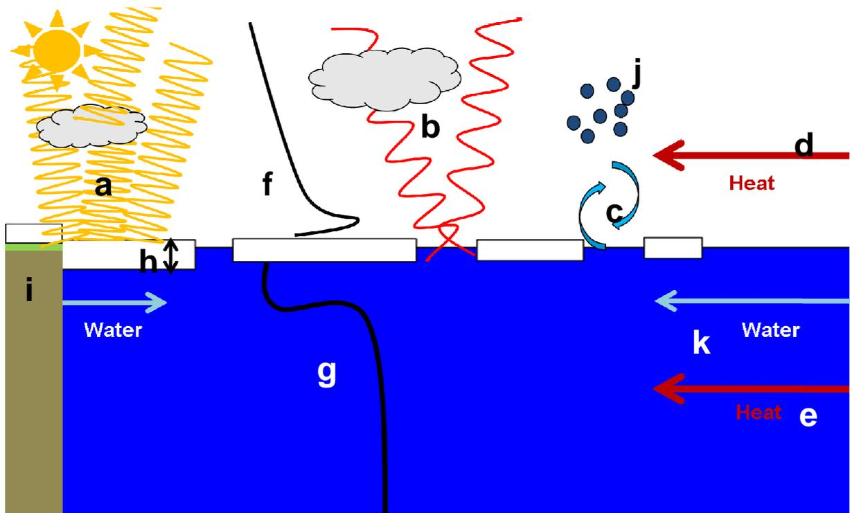
**Figure 1: Key processes governing Arctic climate. a) Net shortwave (SW) solar radiation (modulated by scattering of radiation by clouds and surface albedo) b) Net longwave radiation emitted by surface and by clouds c) Turbulent (sensible + latent) fluxes d) Atmosphere heat transport e) Ocean heat transport f) Atmosphere temperature profile g) Ocean temperature/salinity profile h) Sea ice, thickness and extent i) Land surface processes j) Precipitation k) Freshwater flux e.g. from rivers.**
