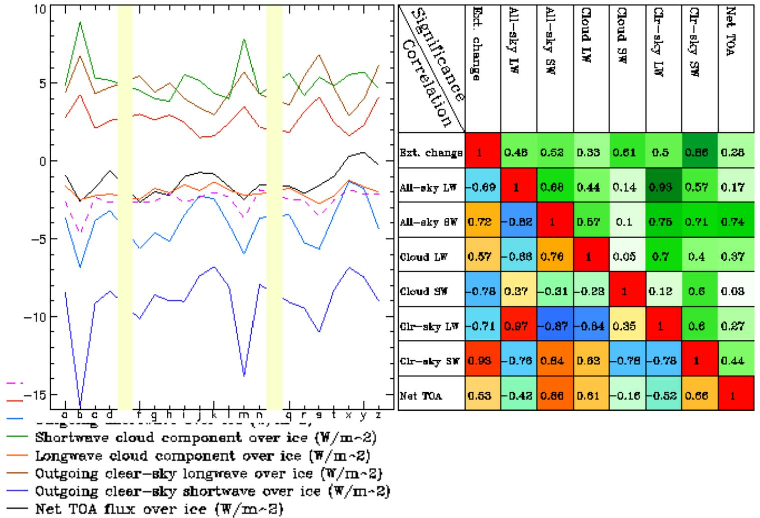
Figure 1. Energy fluxes at TOA, (mean of control experiment yrs 61-80) – (mean of 1% CO<sub>2</sub>/yr experiment yrs 61-80). The change in ice extent is shown also on the same scale: here the mean ice concentration across the 20 years was taken and the area of grid cells of >0.15 concentration taken. LH graph shows the values across the individual ensemble members (a to t) of THCQUMP; the RH table shows the correlations between the quantities.
