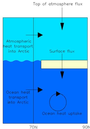
**Figure 4:** Relationship between surface fluxes and heat transport. Atmospheric heat transport into the Arctic ( $T_a$ ) is balance by surface ( $N$ ) and top of the atmosphere ( $R$ ) fluxes ( $N=T_a+R$ ). Ocean heat transport into the Arctic ( $T_o$ ) is balanced by surface fluxes and ocean heat uptake ( $dQ/dt$ ) ( $dQ/dt=T_o+N$ ).
