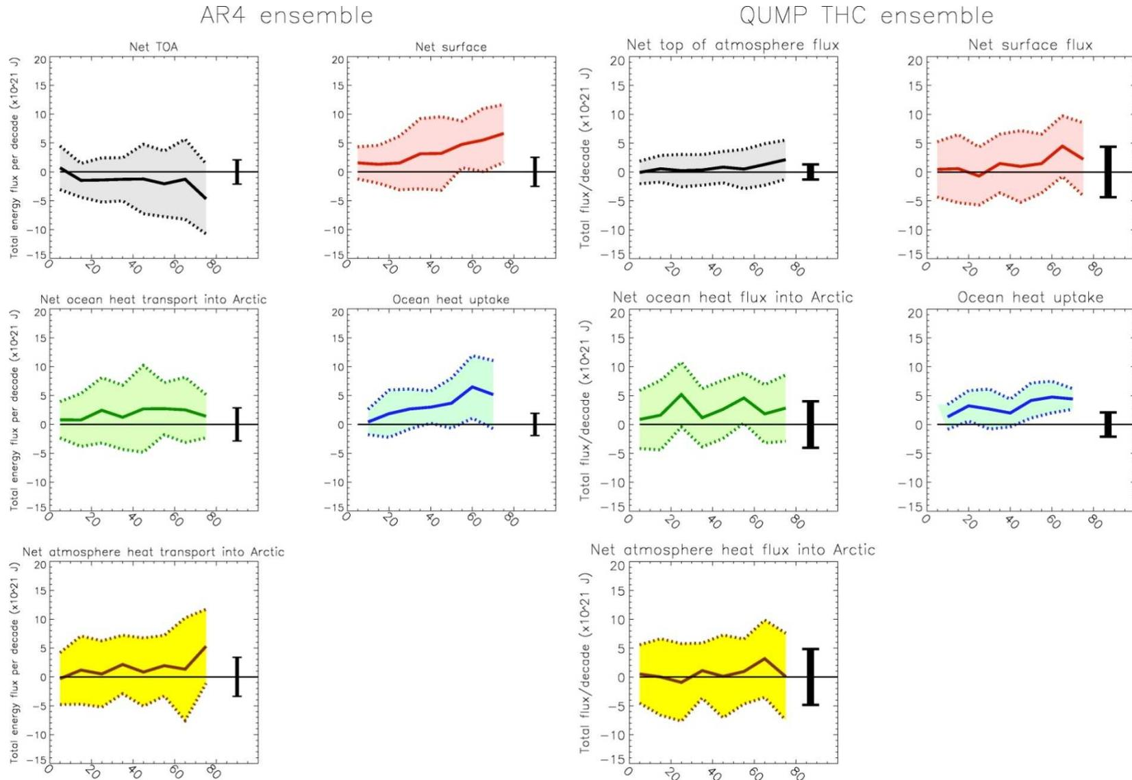
Figure 6: Change in heat budget components for AR4(left) and THC-QUMP(right) ensembles. The coloured shading marks 1 standard deviation of the ensemble. Terms of the heat budget in the two ensembles (decadal means), change from control to 1% experiment. The ensemble mean,  $\pm$  one standard deviation, is plotted, evolving in time. The black bars on the right show RMS (interdecadal standard deviation) across the ensemble.
