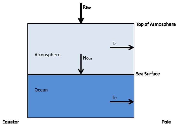
**Figure 9: Schematic to show how the atmospheric and oceanic heat transports ( $T_A$  and  $T_O$ ) are calculated. The net top of the atmosphere radiative fluxes ( $R_{Top}$ ) and the net surface fluxes ( $N_{Ocn}$ ) are defined as positive downward. Northward heat transports are positive.**
